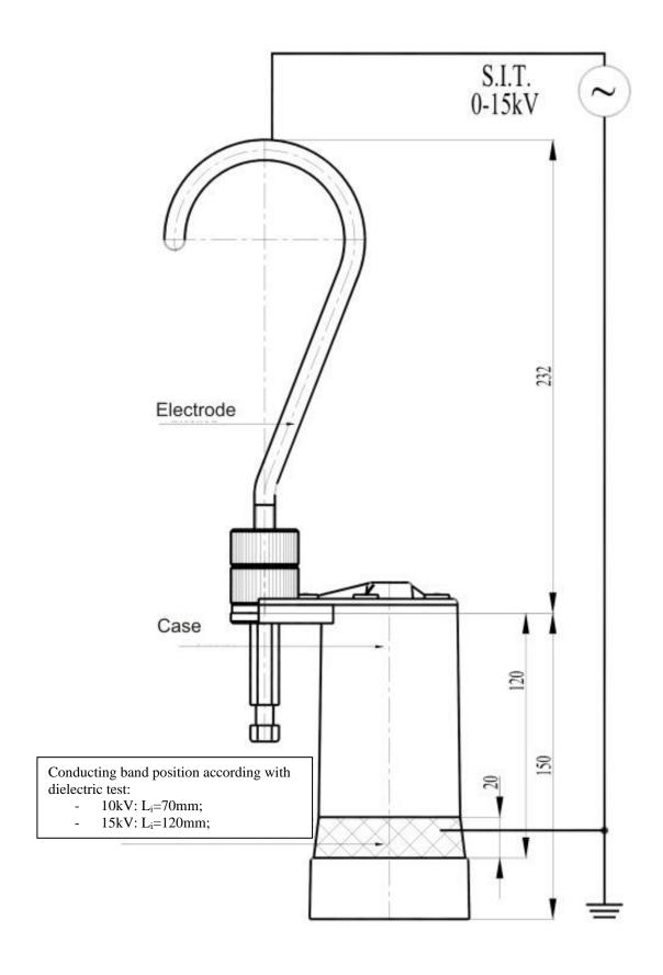
The mounting for the dielectric rigidity test of the case - for voltage detectors DTCIER 110 kV, DTCIER/P 110 kV and DTCIER/P 220-400 kV
