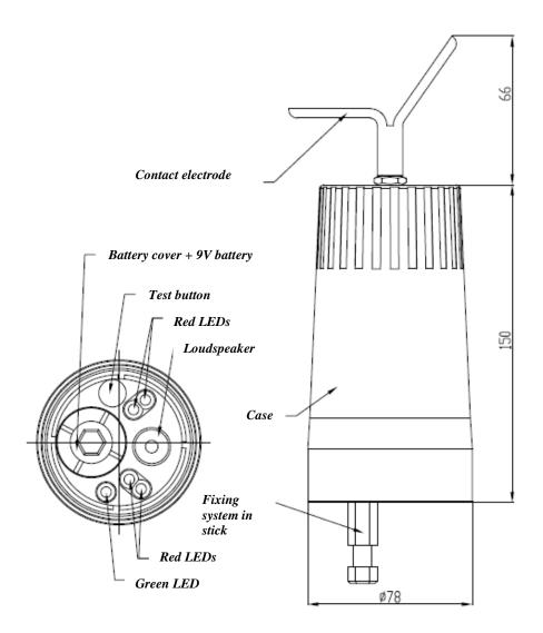
Annex 2 The general appearance of DTCIER 110 kV, DTCIER/P 110 kV and DTCIER/P 220-400 kV detectors
