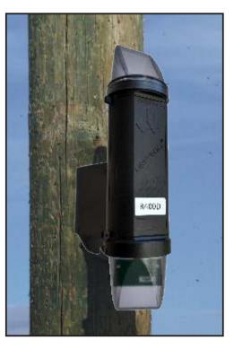
LineTroll R400D continuously monitors the line voltage and current, and detects faults either when the current exceeds an absolute configurable threshold or variation in current within a specific time (di/dt). The units has a built-in load current compensator which allows for detection of very low phase-to-earth faults. The unit has inrush current filtering to avoid false indication when line is energized.
