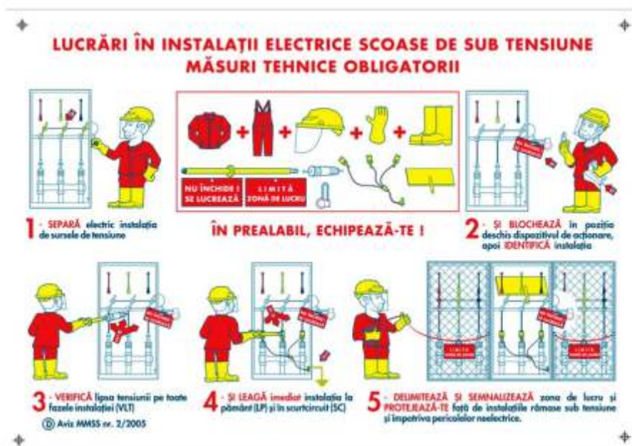
All - "Works on de-energised electrical installations - Five golden rules."
