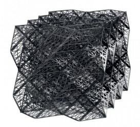
The alternation of the individual elements in the volume of R80 filling can be done in various ways, the most common being the one where the constitutive elements are placed one beside the other, without any distance between them, with the plies of adjacent elements alternatively crossed. In this case, the channels between the constitutive elements have a more complex form, but large enough in order to assure a big air flow through the installation (activation of drought).
